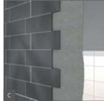
Finally tile, or alternatively apply plaster.
