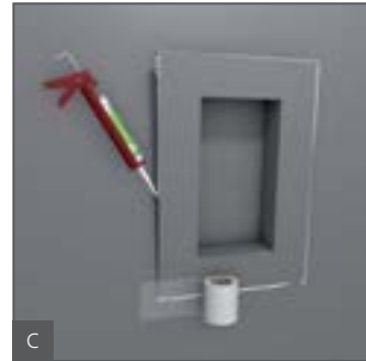
C Add wedi 610 adhesive and sealant and wedi Tools joint reinforcement tape all round it.
